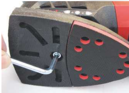
Bases are speedily swapped via a hex key
